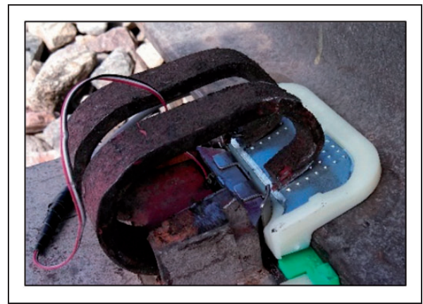
Figure 4. LLED installed in a Safelok I fastening system.
