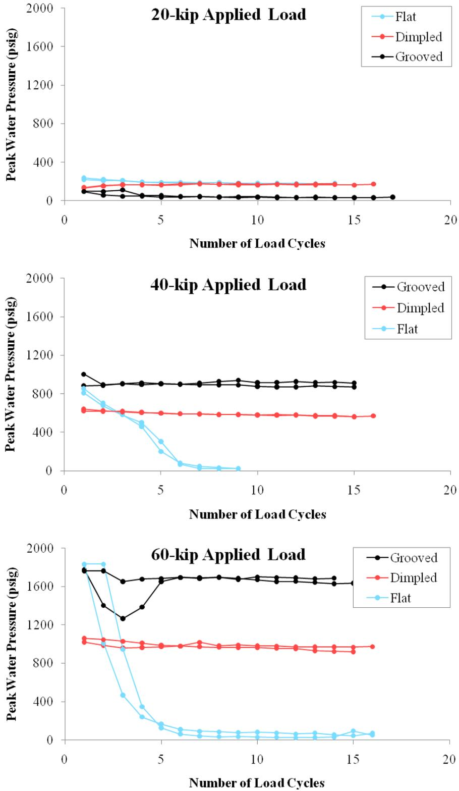
**FIGURE 6. Results of load tests on three different polyurethane pads using square waveform and 6-inch water level**
