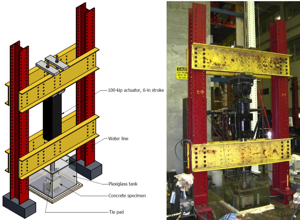
**FIGURE 4. Test setup with a servo-hydraulic actuator loading a concrete block specimen in a water tank**
