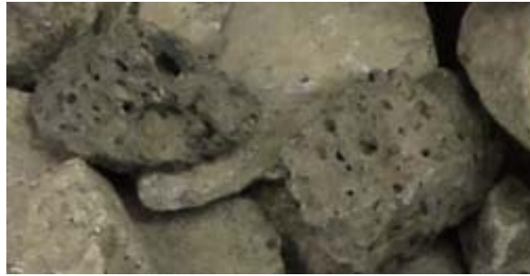
Figure 10 RR 1 Ballast Aggregates with Porous Surfaces
