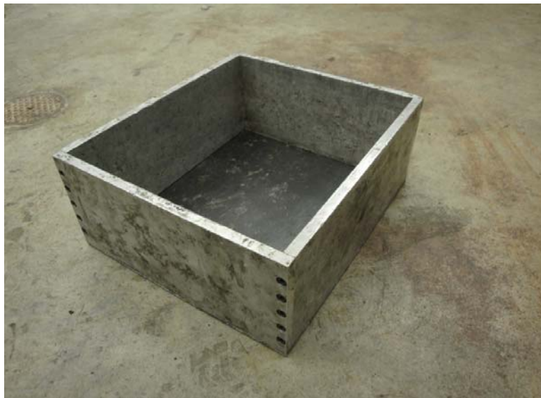
Figure 9 Metal Box Used to Measure Field-Compacted Aggregate Weight to Determine Field Compaction Condition (density or void ratio)
