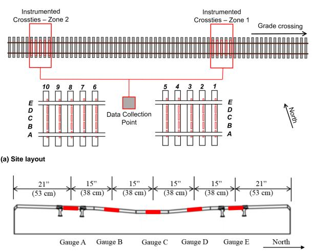
(b) Strain gauge placement map FIGURE 1 Experimentation plan To relate the measured strains to a bending moment, calibration factors were determined by instrumenting three sleepers of the same model and vintage (a representative Class I standard sleeper manufactured in 1997) as those installed in track with the strain gauge layout shown in Figure 1b. A known bending moment was applied to the sleeper and the corresponding strains were recorded to determine the calibration factor.
