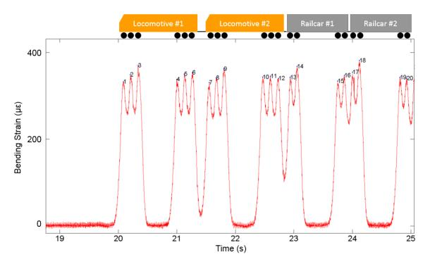
FIGURE 2 Typical strain signal captured under the passage of a loaded train
