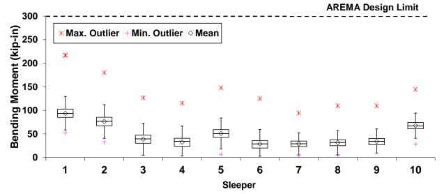
(c) Gauge E (rail seat positive bending moment) FIGURE 3 Box-and-whisker charts of measured bending strains
