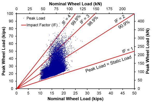
FIGURE 2 Relationship between peak and nominal wheel loads of commuter railcars on Amtrak Infrastructure at Edgewood, MD, Marcus Hook, PA, and Mansfield, MA (WILD data from 2010 and 2011) and design impact factors.
