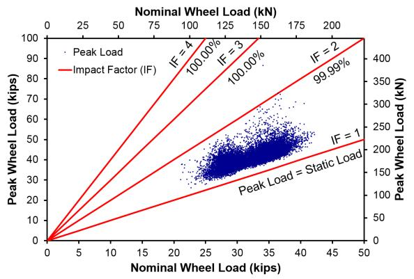
FIGURE 3 Relationship between peak and nominal wheel loads of commuter locomotives on Amtrak Infrastructure at Edgewood, MD, Marcus Hook, PA, and Mansfield, MA (WILD data from 2010 and 2011) and design impact factors.
