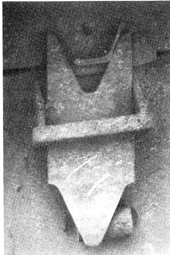
(c) Insulator Broken, Clip Displaced
