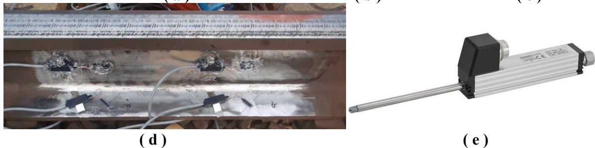
FIGURE 4 Instrumentation used at the MetroLink site: (a) concrete surface strain gauge, (b) laser-based distance measurement device, (c) thermocouple, (d) rail-mounted strain gauges, vertical (above, on rail web, with first layer of protection) and lateral (below, on rail base) (e) linear potentiometer.
