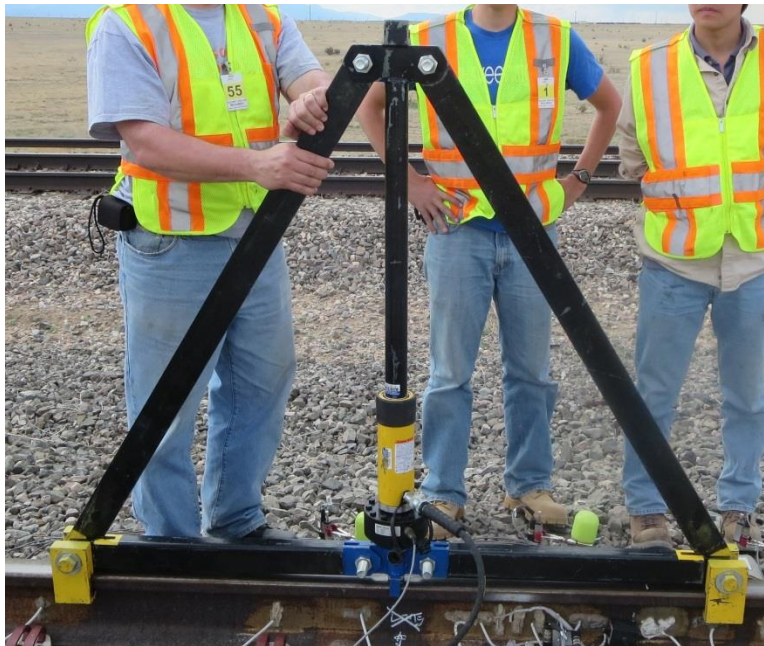
9 10 FIGURE 6 Delta frame used to calibrate strain gauges used to 11 determine vertical wheel-rail input loads. 12
