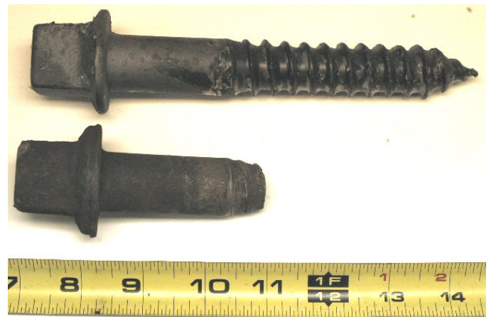
Figure 1. Overview of new and failed screw spikes.
