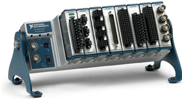
Fig. 2. Compact Data Acquisition (cDAQ) chassis with interchangeable modules [38].
