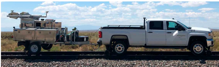
Figure 1. Hi-rail pick-up truck pulling hi-rail test trailer.
