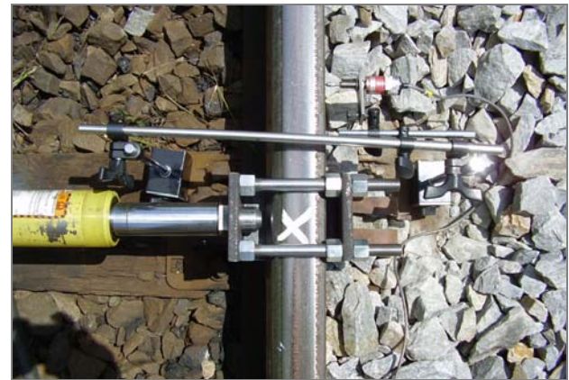
Figure 6. TPCI's Rail Rollover Restraint Fixture
