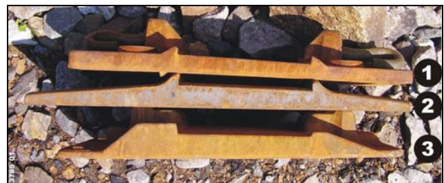
Figure 2. Profile View of the Three Fastening System Tie Plates installed: (1) NorFast, (2) NS-Standard, (3) AirBoss
