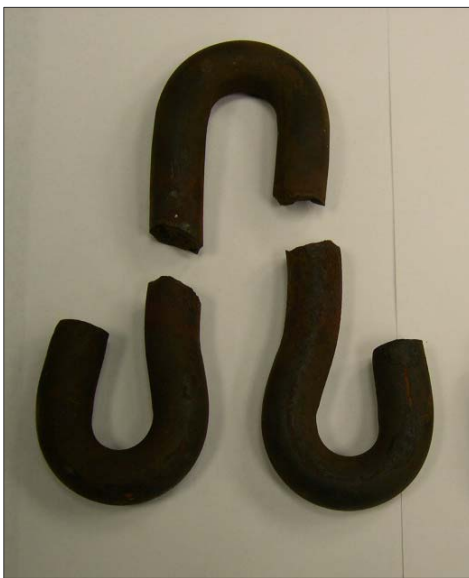
Figure 6. Parts of a NorFast Rail Clips Fractured at 70 MGT
