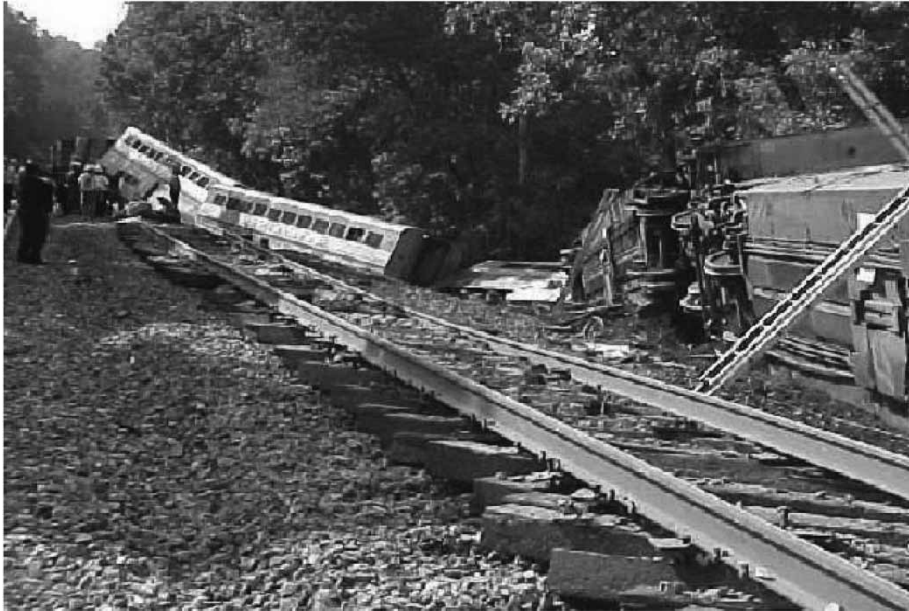
Fig. 1 An example of problems due to voided support
