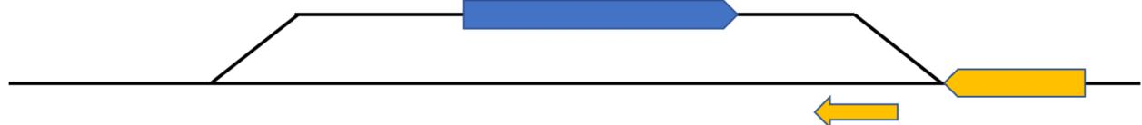
**Figure 2: Lower priority train (blue) stopped in a passing siding while waiting for higher priority train (orange) to pass in other direction**
