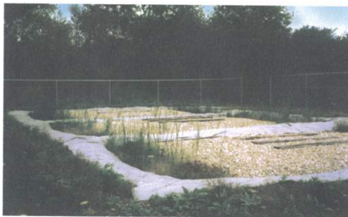
Figure 1: Railway tie study mesocosm as it appeared in November 1998. Three treatments included new and used creosote-treated railway ties plus untreated control ties. The vegetation community growing within the constructed wetland area adjacent to the ballast is dominated by wetland species.
