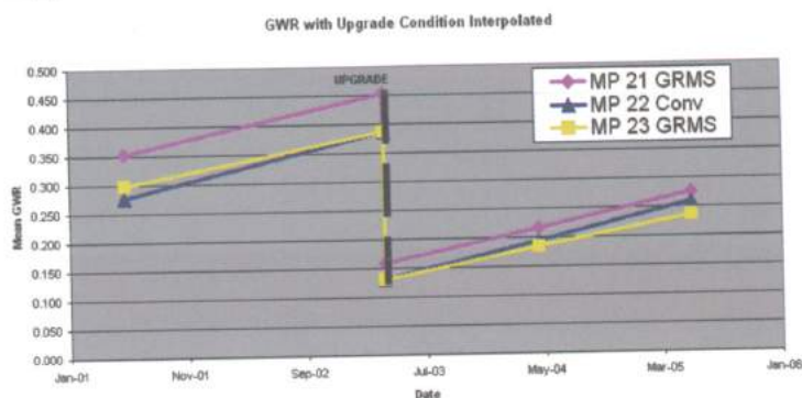
Figure 2: Mean GWR as a Function of Traffic and Upgrade
