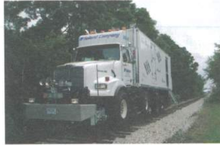
Figure 4B: TrackStar Hi-Rail Inspection Vehicle 3
