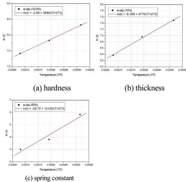
Fig. 3 Change of characteristics for rail pad after heat aging
