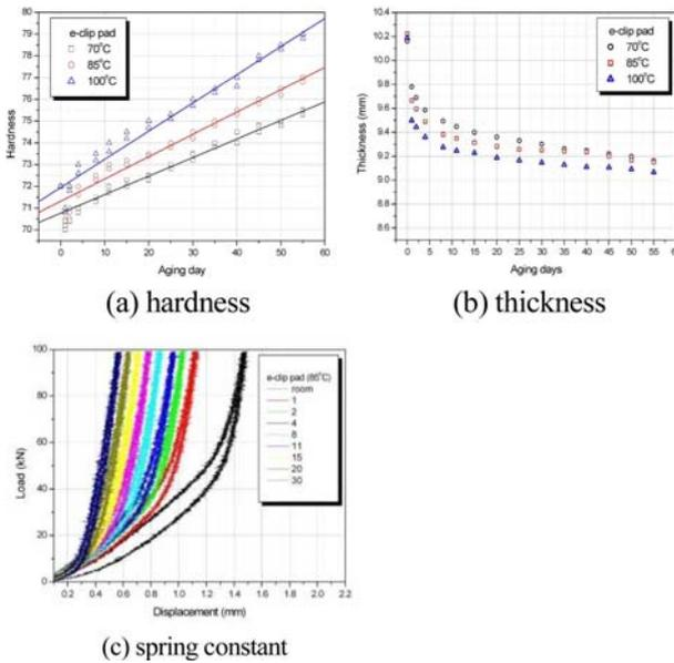
Fig. 2 Mechanical test of rail pad
