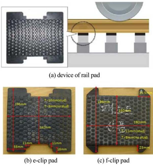
Fig. 1 Rail pad for high speed railway vehicle
