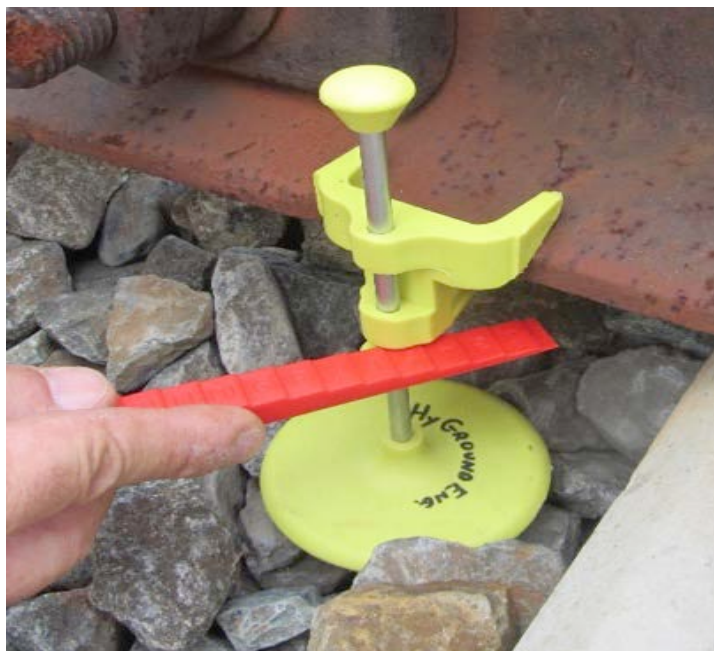
Measurement of Voids Underneath Ties Using Void Meters
