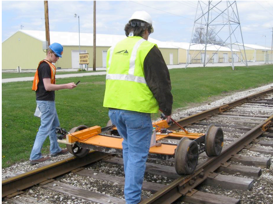
A: Video Track Cart in Use on Low-Density Track
