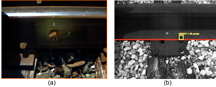
Figure 2: VTC Lighting Setup: (a) Handheld Camera Image of Light Illuminating the Web of the Rail, (b) Lateral View Image Showing Successful Measurement of Raised Spike Using Illuminated Image Captured from VTC
