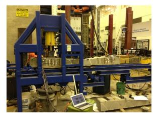
FIGURE 1 STATIC TIE TESTER (STT)
