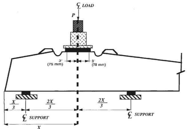
Figure 4. Rail seat positive test
