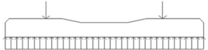
Figure 2. Support assumption for center negative bending [5]
