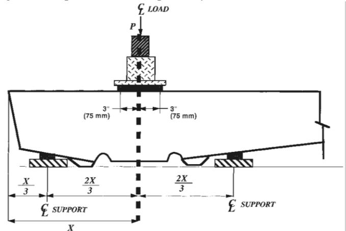
Figure 3. Rail seat negative test
