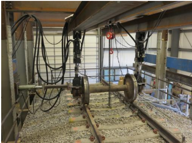
Figure 4. Track Loading System (TLS) Installation during Experimentation
