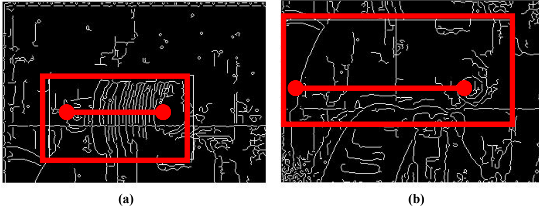
Figure 18 (a) The return spring portion detected, and the amount of compression measured with the red line, and (b) the brake caliper portion detected, and amount of brake application measured with the red line.
