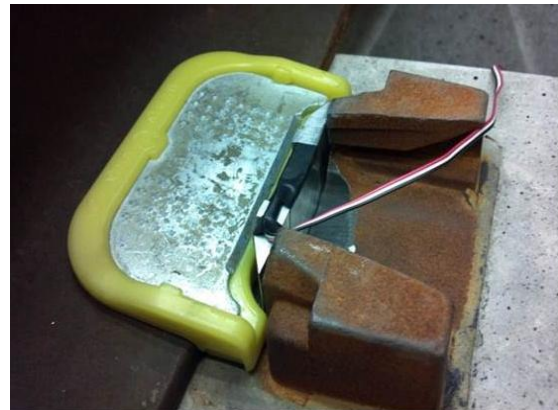
Figure 2 LLED installed on shoulder
