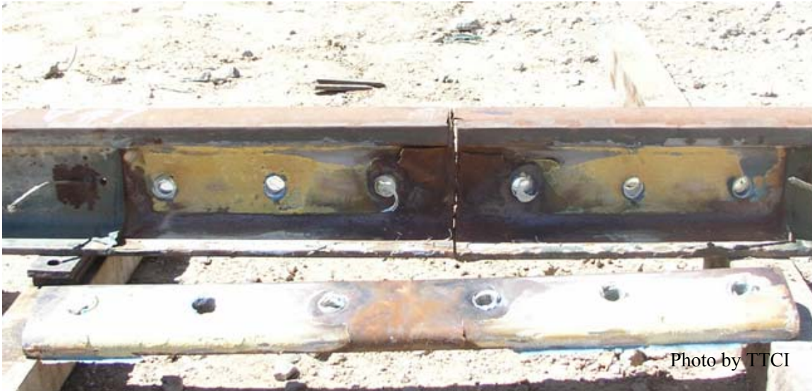
FIGURE 2: Disassembled IJ. Rusty areas show where the epoxy debonded from the metal.
