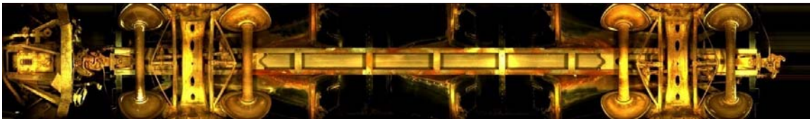
FIGURE 3 Panoramic image of the underbody of a hopper car taken at the Monticello Railway Museum.
