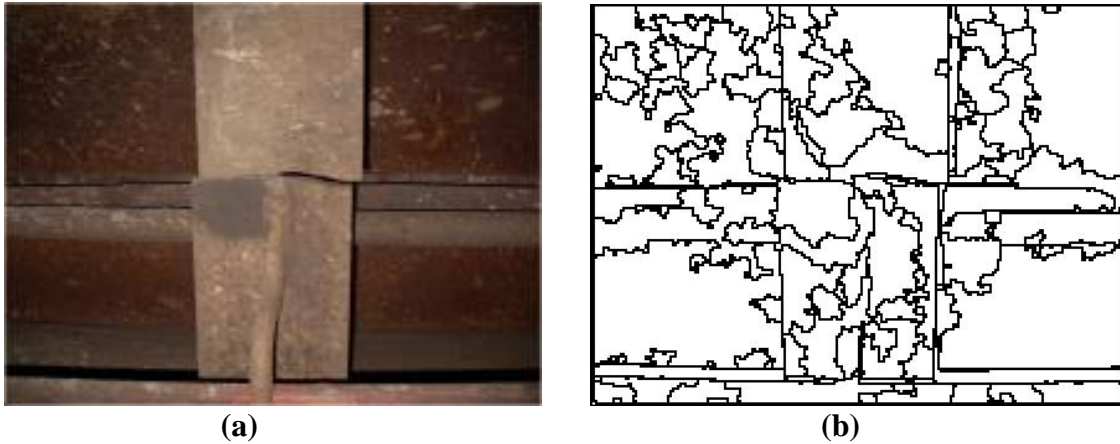
FIGURE 5 (a) Digital picture of a broken crossbearer with (b) a multiscale segmentation of the image.
