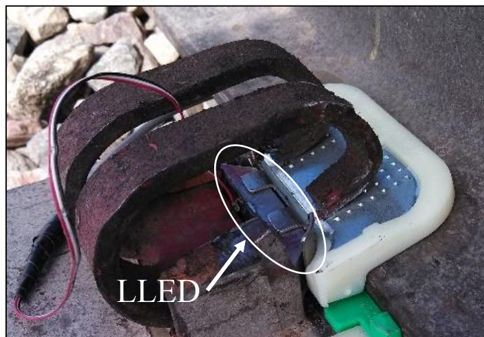
7 8 9 FIGURE 3 LLED installed in Safelok I fastening system.
