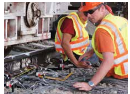
RESEARCH TO MEASURE STRESSES IN THE RAILWAY CROSSTIE FASTENING SYSTEM CONDUCTED BY UNIVERSITY OF ILLINOIS STUDENTS WILL HELP ADDRESS THE CRITICAL ENGINEERING CHALLENGES OF OPERATING HEAVY-AXLE-LOAD FREIGHT AND HIGHER-SPEED PASSENGER TRAINS ON THE SAME TRACK INFRASTRUCTURE.
