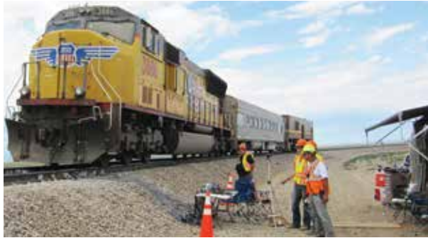
UNIVERSITY OF ILLINOIS RAILTEC STUDENTS AND RESEARCH ENGINEERS UNDERTAKE FULL-SCALE TESTING OF THEIR INSTRUMENTED CONCRETE CROSSTIES AT THE TRANSPORTATION TECHNOLOGY CENTER NEAR PUEBLO, COLORADO.
